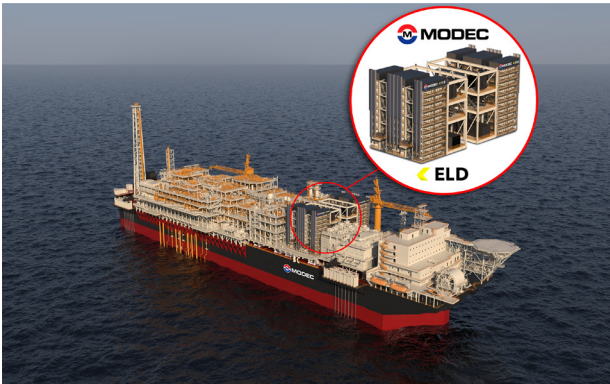
Integrated 100 MW SOFC + CO 2 capture system for FPSOs
