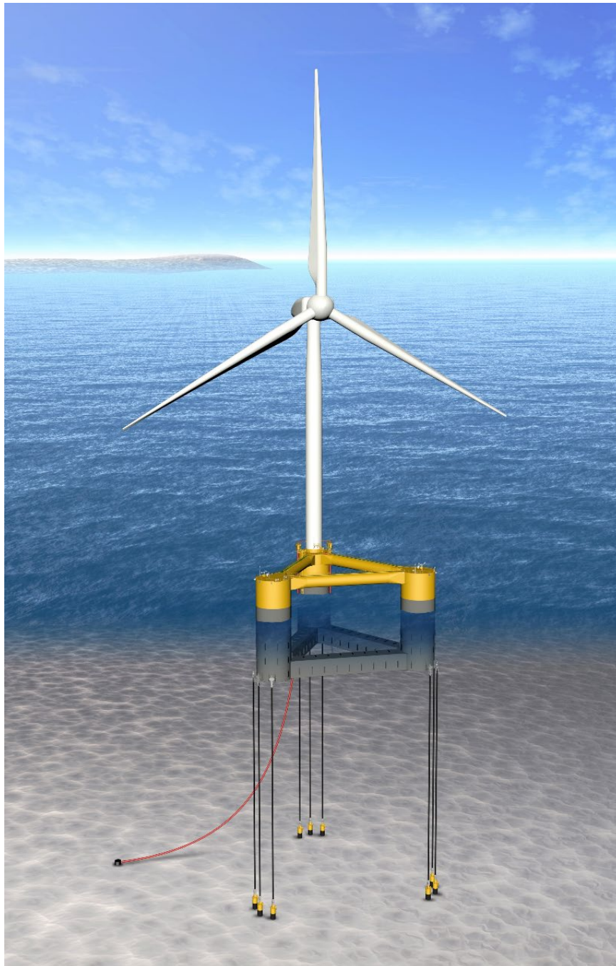
Conceptual drawing of TLP (Tension Leg Platform) [Source: MODEC]
