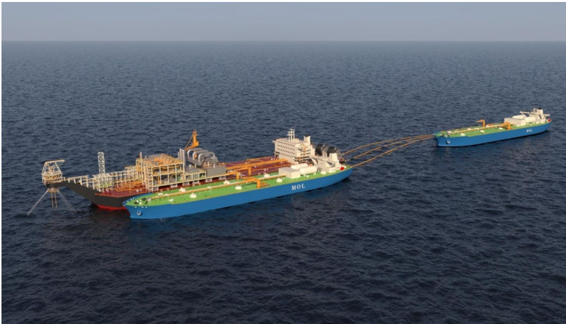
MODEC LCO 2 FSIU, showing dual offloading to MOL LCO 2 Carriers
