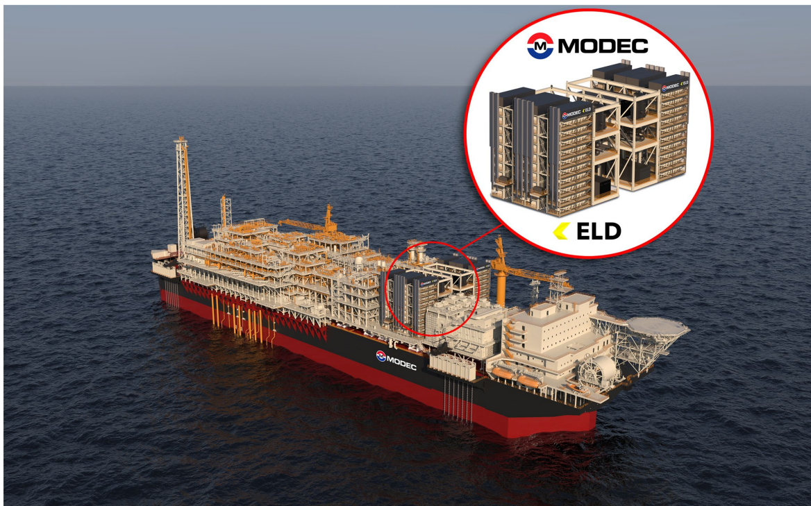
Conception Illustration of FPSO with full scale (100 MW) SOFC installation with integrated carbon capture.
