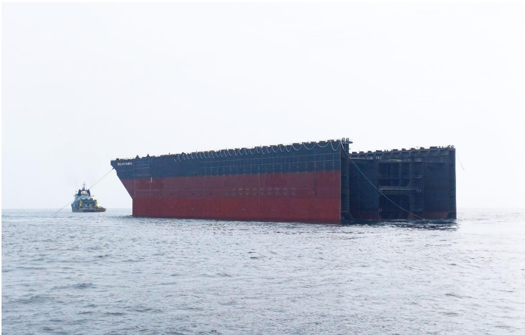
Forward Section of MODEC’s Next Generation Hull for FPSO Gato do Mato
